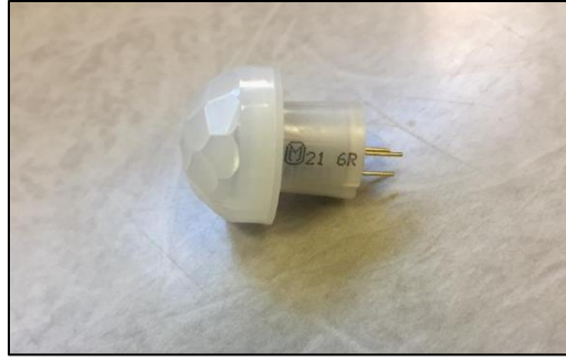
Figure 1. Panasonic AMN24112 device used in both novel PIR systems introduced in this work
