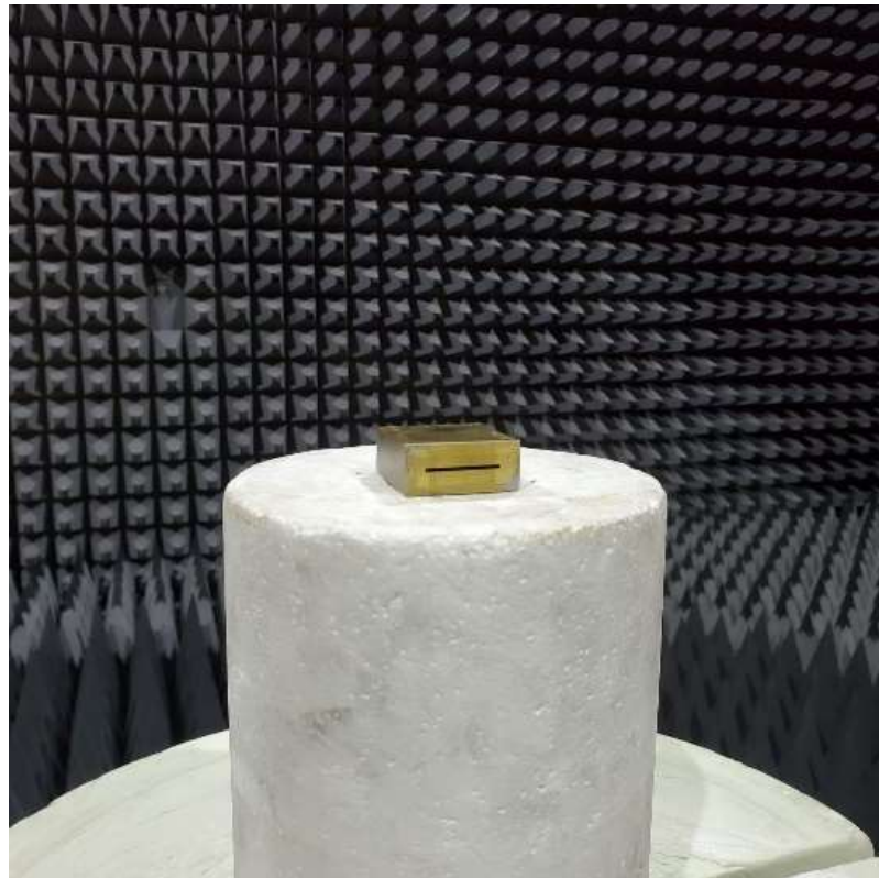
Figure 4.3. V2X cavity-backed slot antenna measured on foam inside anechoic chamber.
