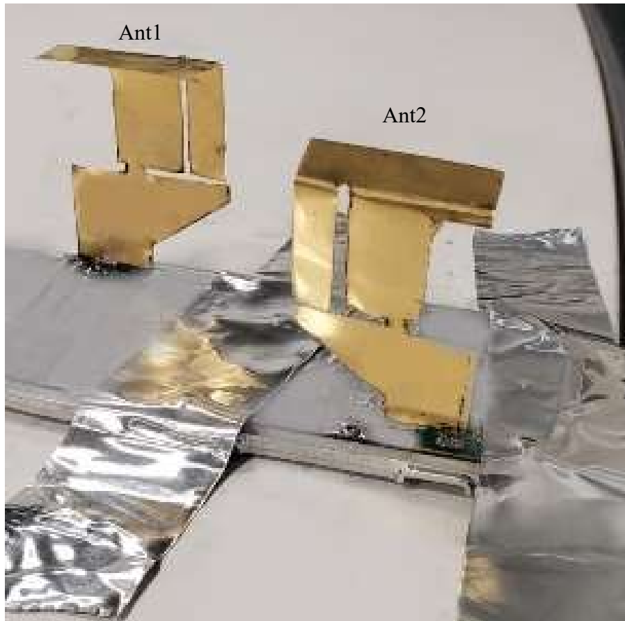
Figure 3.2. Configuration I of a 2x2 5G MIMO system placement on vehicle roof.
