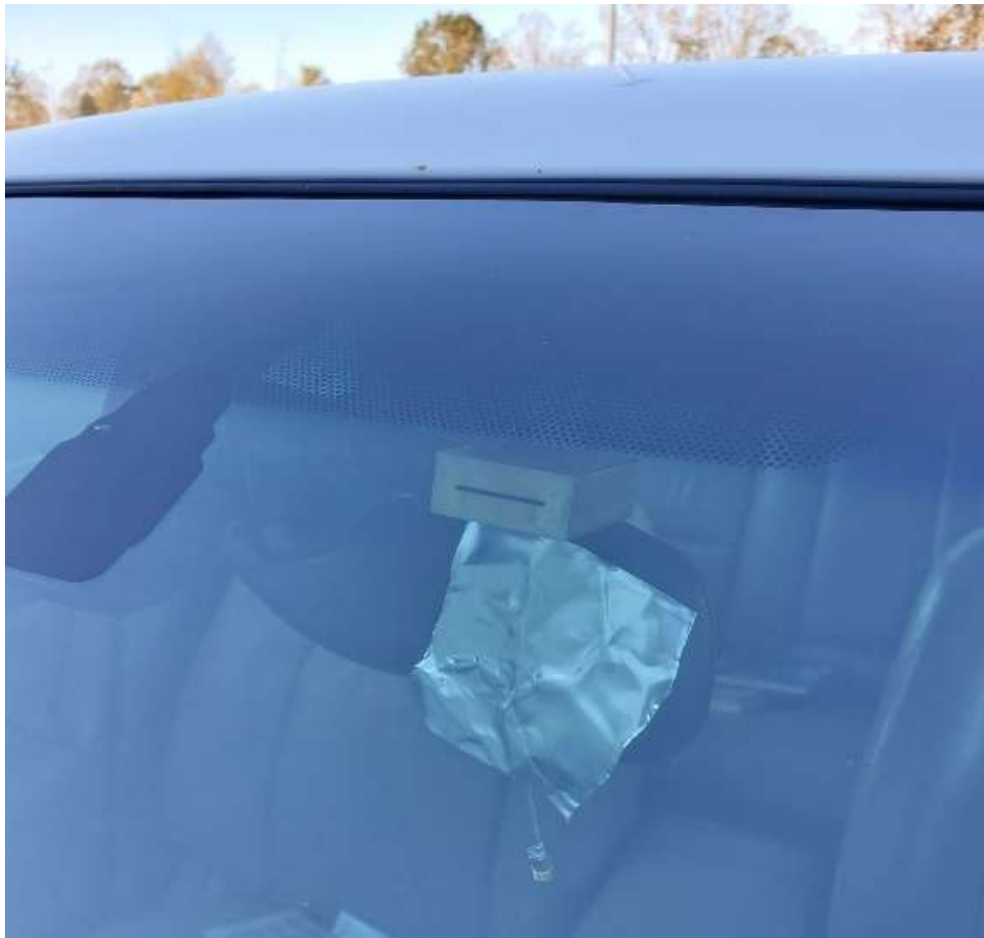
Figure 4.4. V2X cavity-backed slot antenna mounted on vehicle's windshield ready for chamber measurement.
