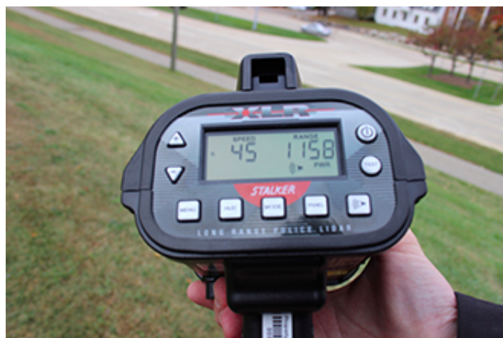
The LIDAR device measures a target's speed and distance.
