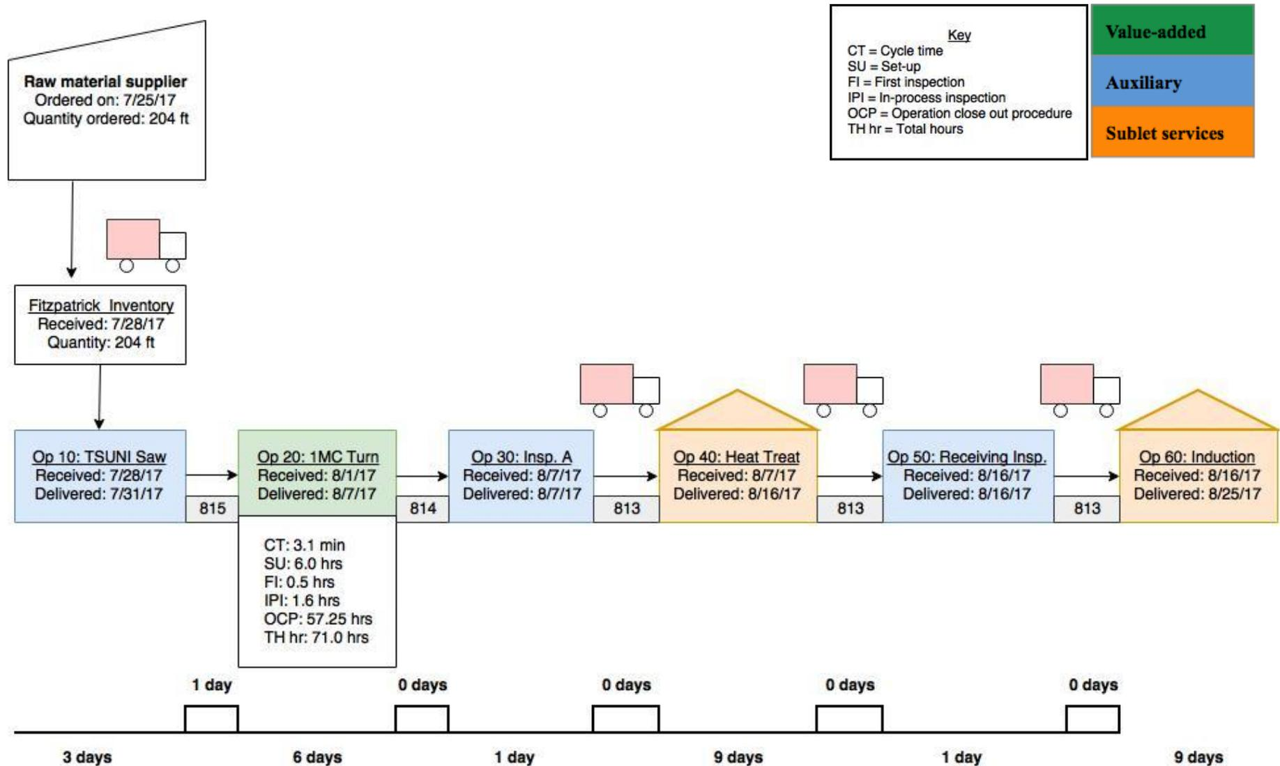
Figure 3.2: Value stream map of FMC’s slip-wicker manufacturing process (Part two)
