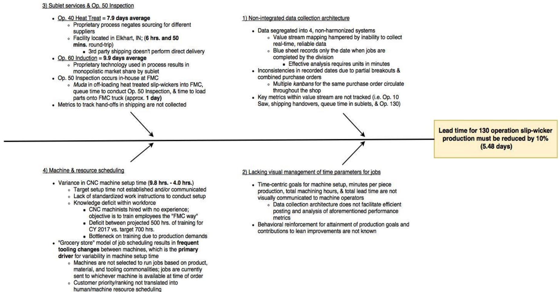
Figure 10: A3 report - Lead time reduction for slip-wicker manufacturing kaizen
