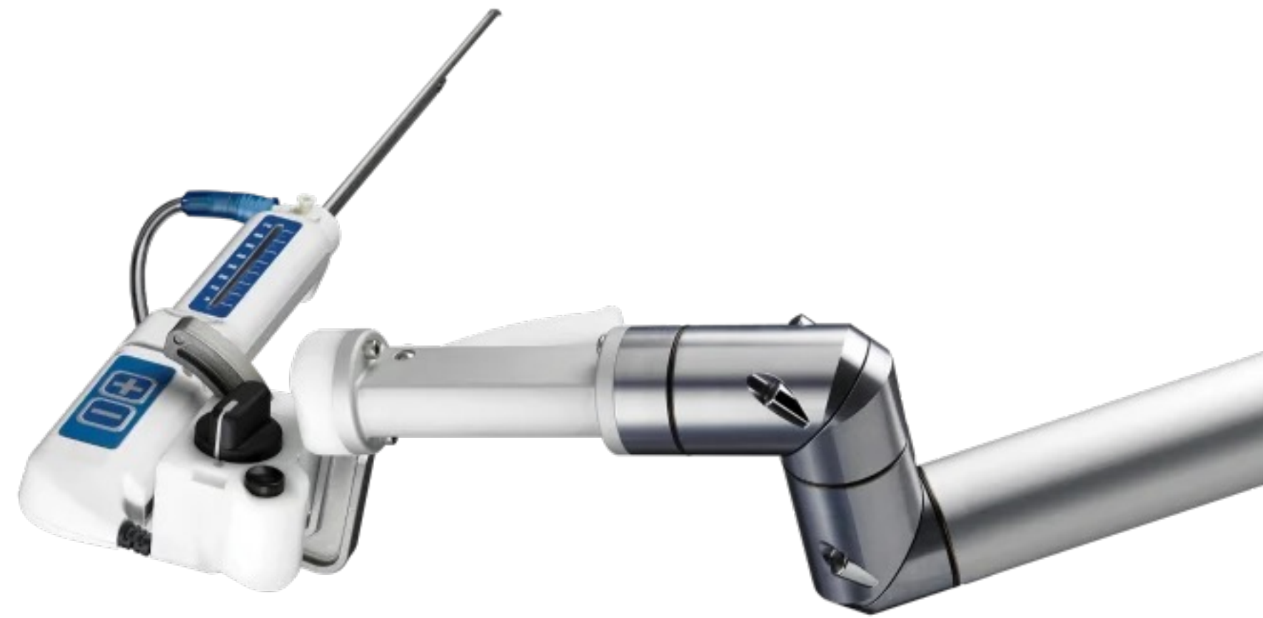
Figure 1. Aquablation handpiece with robotic arm. The Aquablation system utilizes a robotic-assisted waterjet under ultrasound guidance to precisely resect prostate tissue for the treatment of BPH. 7
