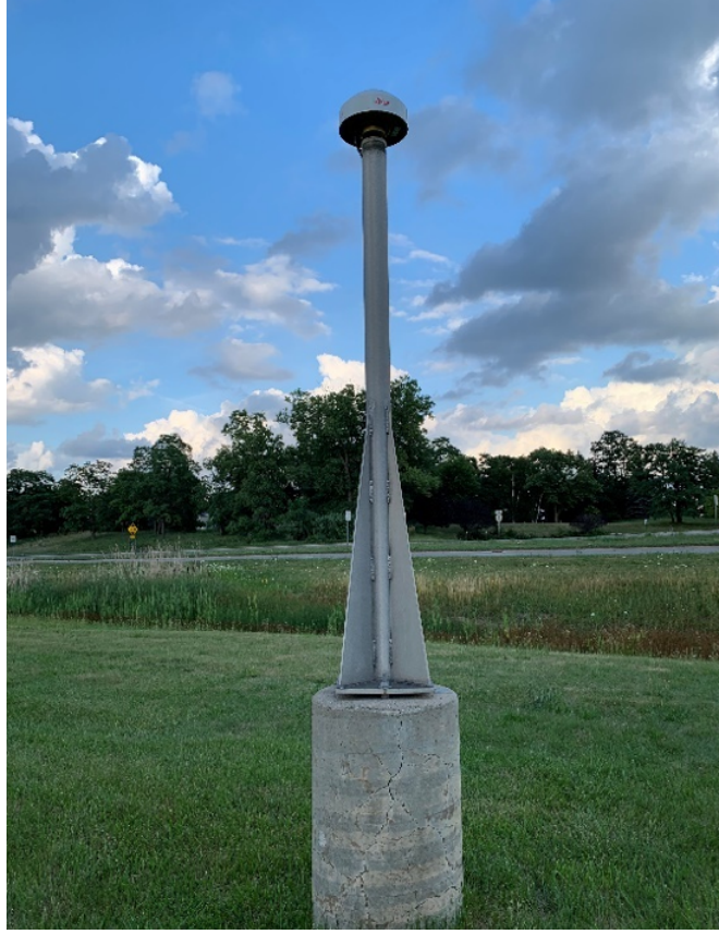
Figure 3.27: Reference observation station setup with receiver and antenna
