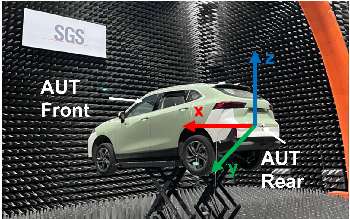
Figure 4.6: On-vehicle testing under MVG-SG 3000 full-scale chamber
