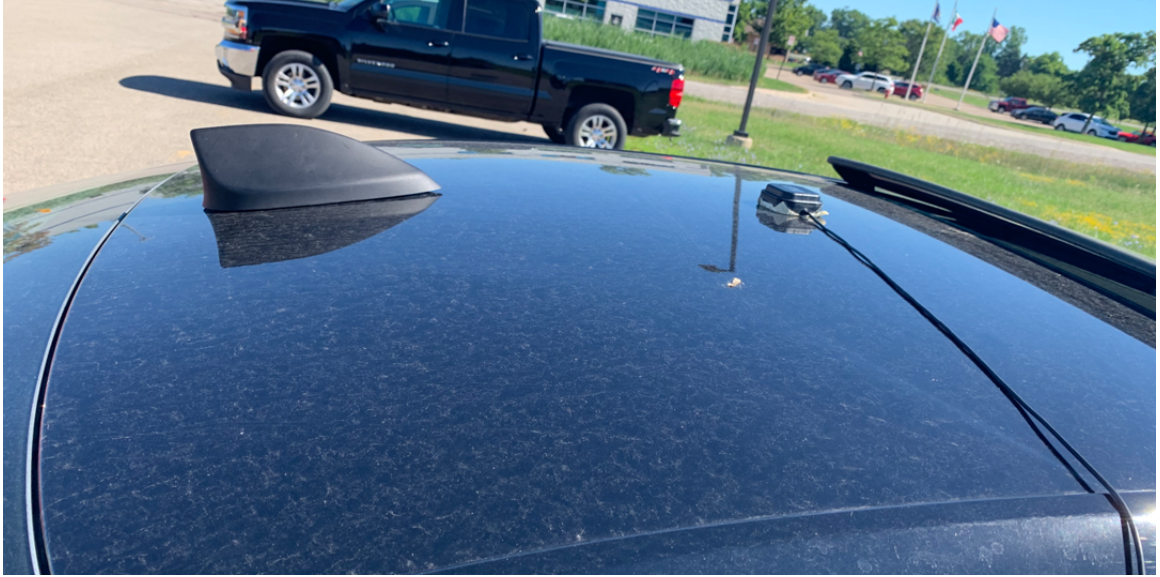
Figure 3.30: User shark-fin GNSS L1/L2/L5 band antenna setup
