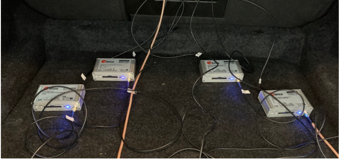
Figure 3.31: u-blox receivers setup on-vehicle
