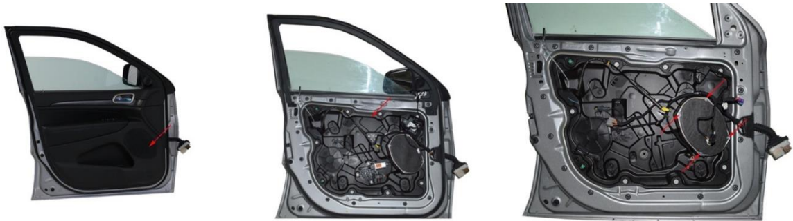
Figure 7.1 Typical door speaker system location (left), door carrier module (middle), and speaker attachment points (right)
