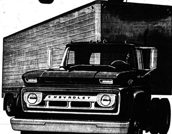
New SERIES 80 DIESEL. Diesel savings and sure Chevy durability. New 17,000-lb. hypoid rear axle now available on D80-H models.
