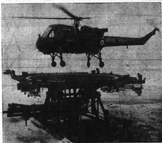
GETTING SEA LEGS ON LAND—A British naval helicopter descends for a landing on a rocking platform at the Royal Aircraft Establishment at Bedford, England. The platform, which can be tilted several degrees in any direction, was built to simulate the pitching and rolling action of a ship at sea.
