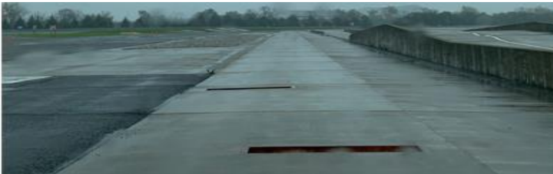
Figure 5.2: controlled proving ground test tracks used to generate deterministic vehicle dynamics disturbances for ground truth labeling
