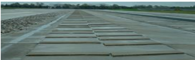
Figure 5.6: controlled proving ground test tracks used to generate deterministic vehicle dynamics disturbances for ground truth labeling
