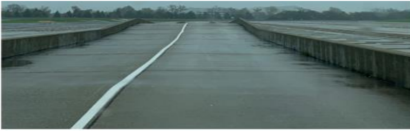
Figure 5.7: controlled proving ground test tracks used to generate deterministic vehicle dynamics disturbances for ground truth labeling
