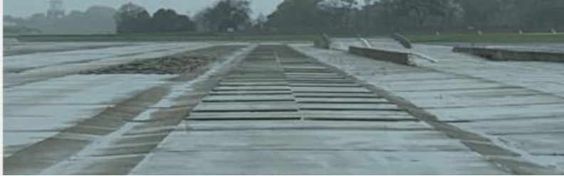
Figure 5.1: controlled proving ground test tracks used to generate deterministic vehicle dynamics disturbances for ground truth labeling
