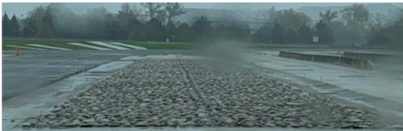
Figure 5.3: controlled proving ground test tracks used to generate deterministic vehicle dynamics disturbances for ground truth labeling
