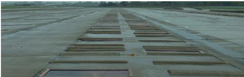
Figure 5.5: controlled proving ground test tracks used to generate deterministic vehicle dynamics disturbances for ground truth labeling
