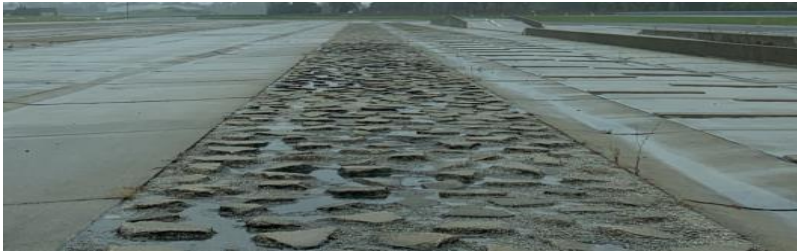
Figure 5.4: controlled proving ground test tracks used to generate deterministic vehicle dynamics disturbances for ground truth labeling
