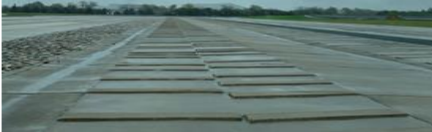
Figure 5.8: controlled proving ground test tracks used to generate deterministic vehicle dynamics disturbances for ground truth labeling
