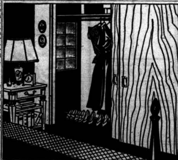
CHECK MOTHS — That dark closet in your home can be as bright as any room in the house if it's located on an exterior wall. A panel of translucent glass block will flood the area with daylight, at the same time protecting the interior from the view of outsiders. In addition to eliminating the inconvenience of darkness, daylight will help to prevent moths. They prefer to work in the dark.
