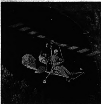
ONE-MAN ROTORCRAFT —A commuter helicopter for the average man may yet become reality as designers continue to simplify the complex and sometimes temperamental craft. This craft, the Benson Gyrocopter, is a combination of helicopter and autogyro features. It has a lifting capacity of 250 pounds, a range of 120 miles and a flight speed of between 15 and 45 m.p.h.
