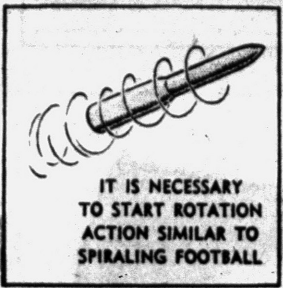
More auxiliary rockets could fire automatically to set up a desirable rotation speed of something like 200 revolutions per minute.
