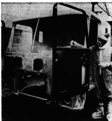
Undercoating Is Applied Prior To Painting
