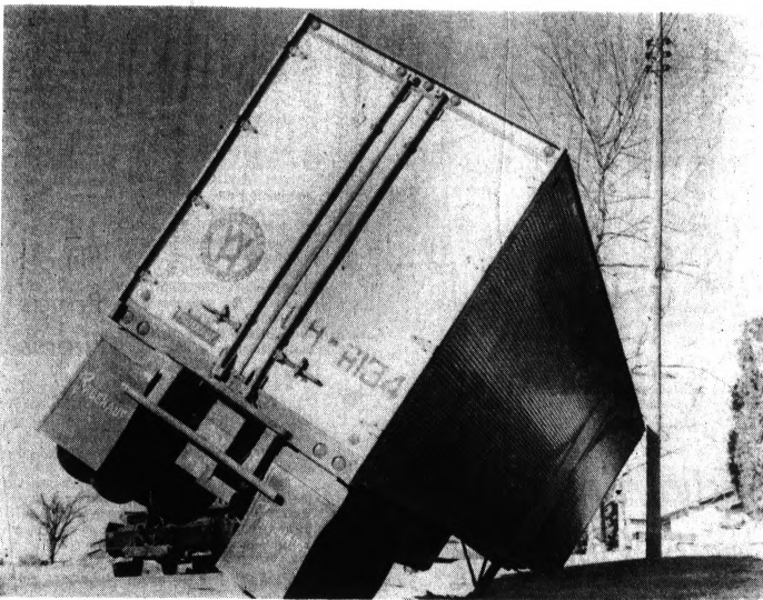
A HITCH IN UNHITCHING — The truck driver who unhitched this trailer did so because he wanted to get the truck repaired. He stood helplessly as the trailer's small front wheels sank in the soft roadside at Alton, Ill. Alton police kept sightseers away and crossed their fingers until a tow truck could right the trailer.
