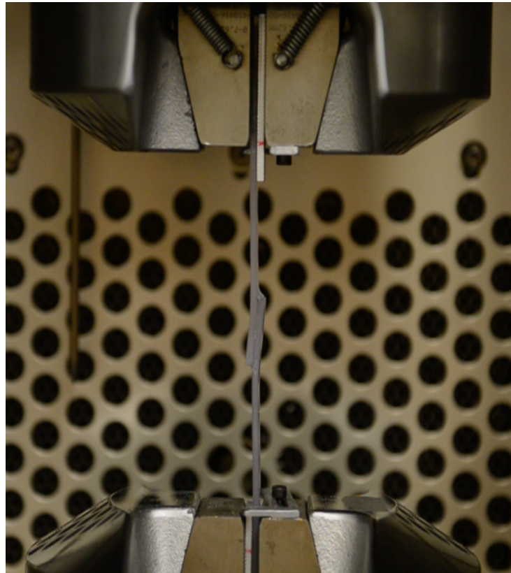
Figure 2.8 Static LTC Test Setup with Polycarbonate Coupon
