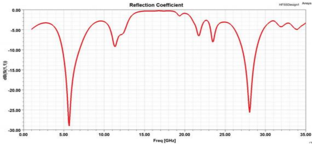
Figure 4. 7: Simulated reflection coefficient ( |S_{11}| ) of the proposed 2 \times 3 bridge-connected multiband MIMO antenna.
