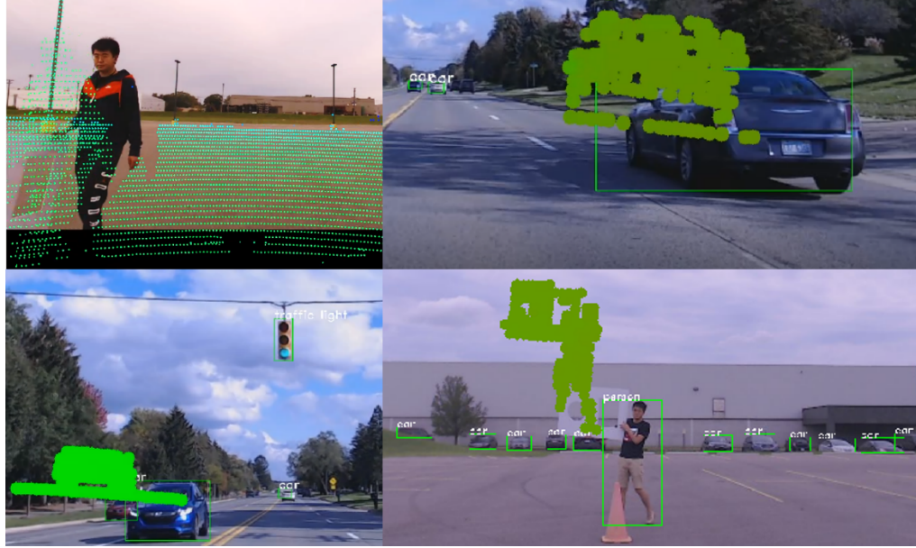
Figure 5.5 Calibration error results in LiDAR-Camera sensor fusion
