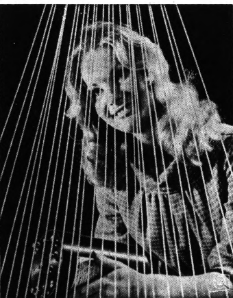
TOP DRAWER —Two miles of metal ribbon such as pretty Marianne Kowalski is peering through is needed to wind the superconductive magnet she is holding. The magnet will be used in high-energy physics experiments in addition to medical and biological research. Engineers for RCA, who developed the magnet, say it has a field strength 200,000 times as powerful as the earth's magnetic field.
