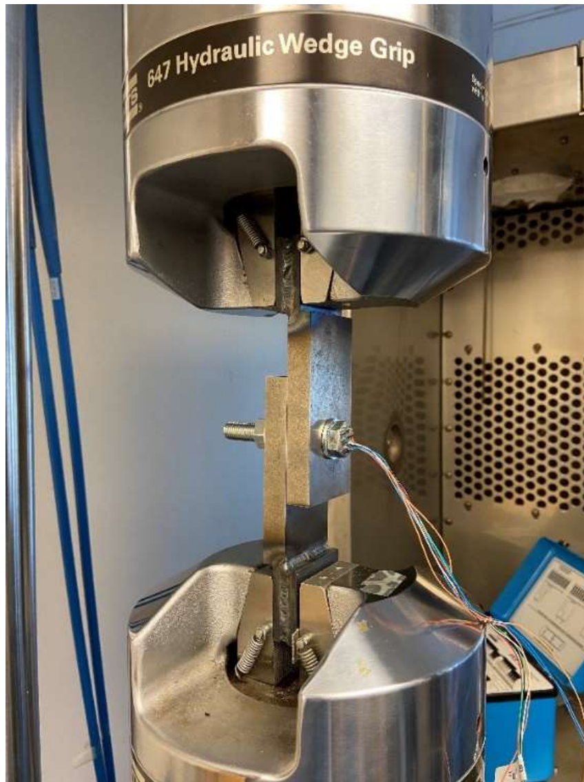
Figure3.5 Shear strain gage calibration.
