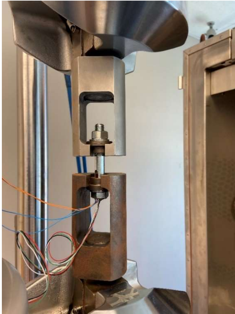
Figure 3.3 Axial strain gage calibration.
