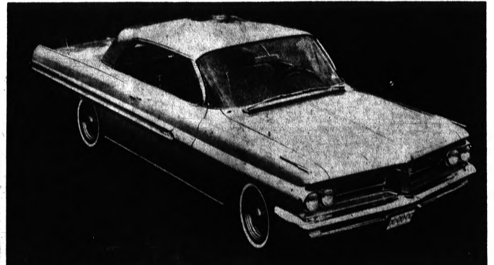
FROM THE FRONT — The new sports car of Pontiac Motor Division, the Grand Prix, is only 54.5 inches high and features Pontiac's proven wide-track wheels. Under the hood are 303 horses housed in a Trophy V8 engine with a four-barrel carburetor.
