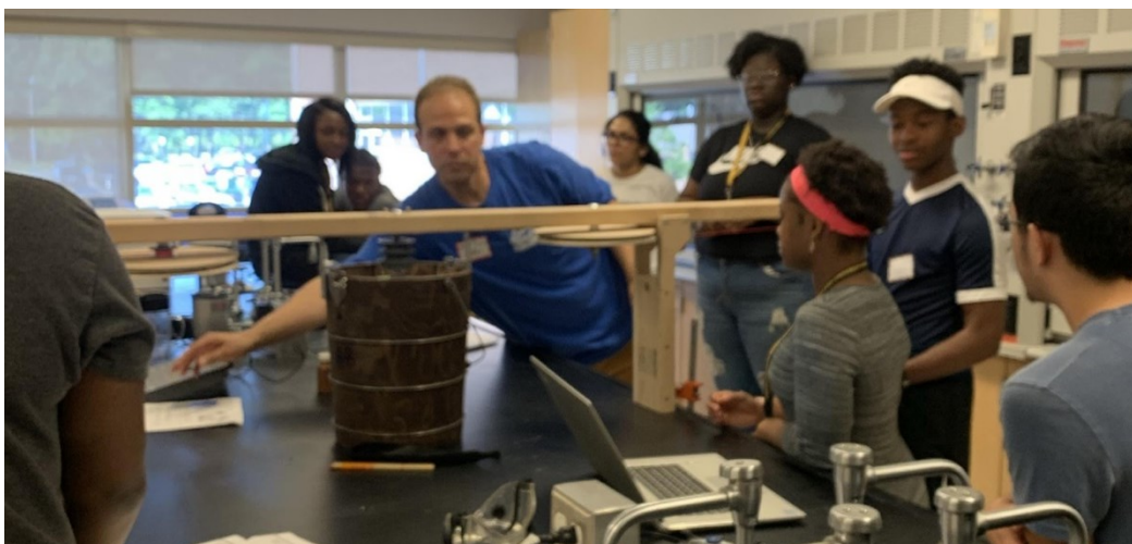
Figure 5.2: Dr. Raffel demonstrates to PUB students how to use the custom-built Joule apparatus to convert mechanical energy into heat energy. Designed to drop two 3 kg weights in succession to spin a paddle in the center bucket filled with water to raise the temperature of the water by adding mechanical energy to the system. Photo credit: Ava McDowell.
