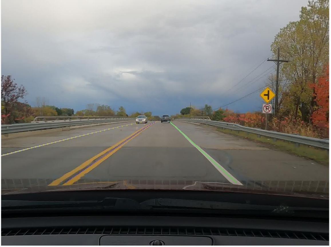
Figure 19 Detected lane markers overlaid on the input image
