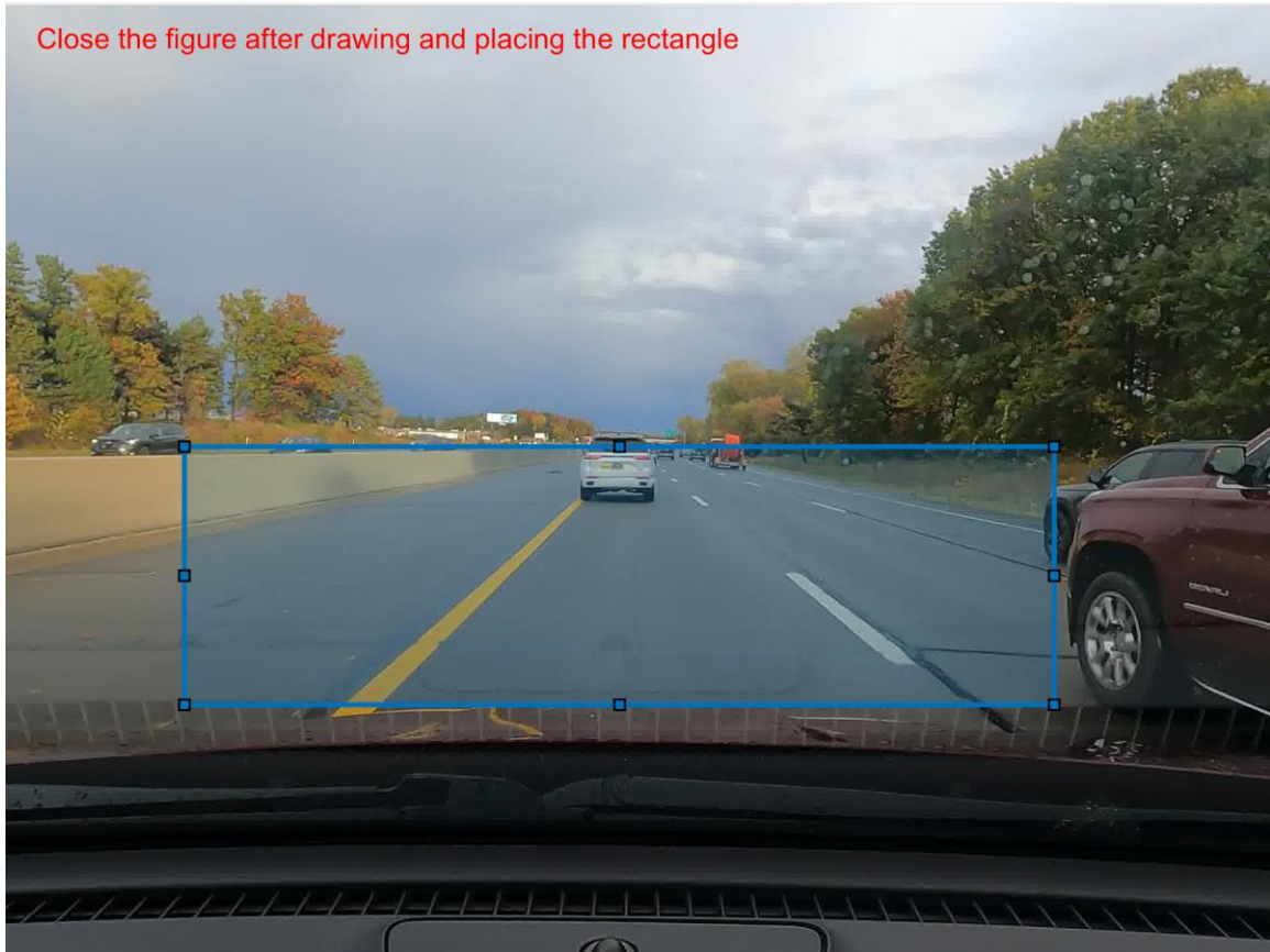
Figure 18 ROI to exclude the skyline from the extraction algorithm
