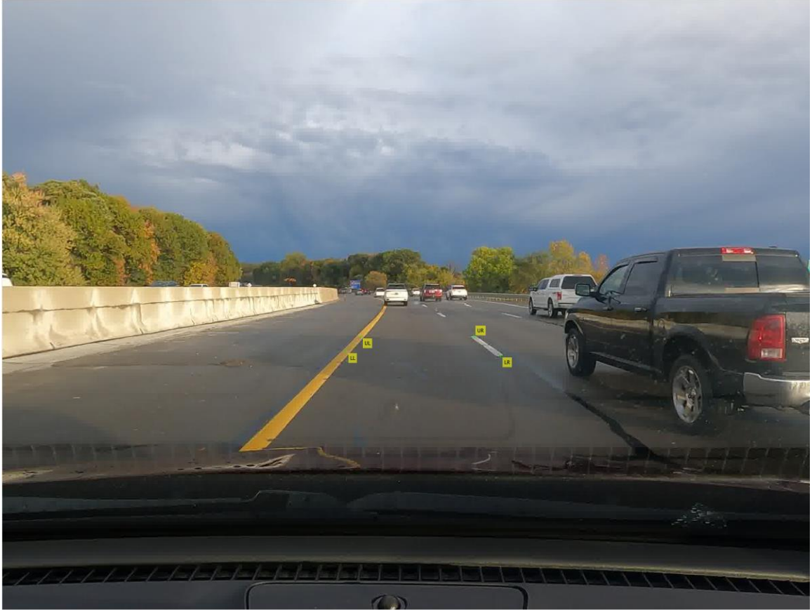
Figure 15 Pixel coordinates of a trapezoid in the scene image for calibration
