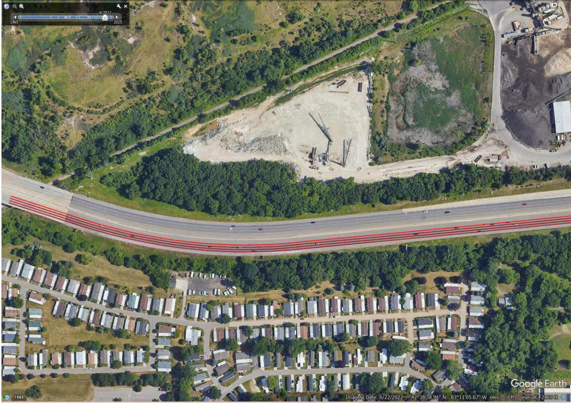
Figure 26 generated lane boundaries on M59 east after fusing vision data with OSM data
