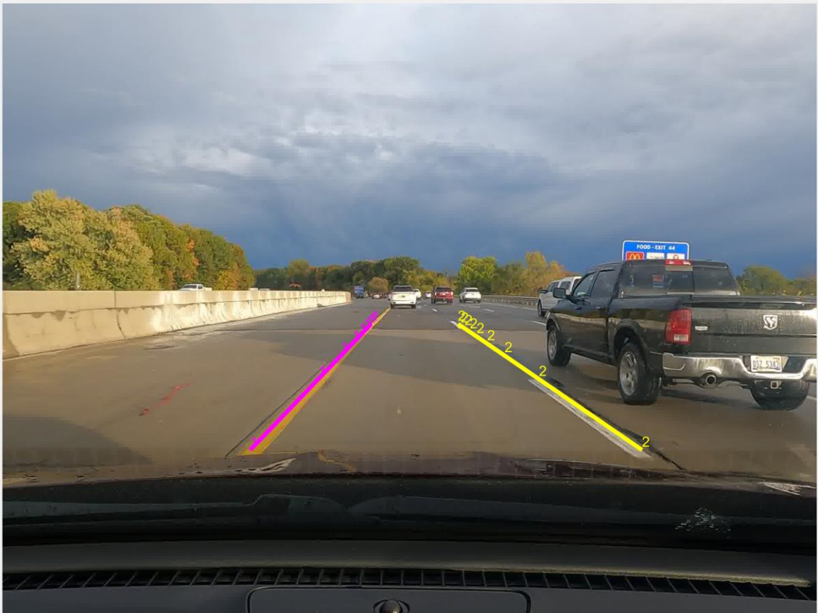
Figure 20 Tracked lane boundaries in vehicle frame
