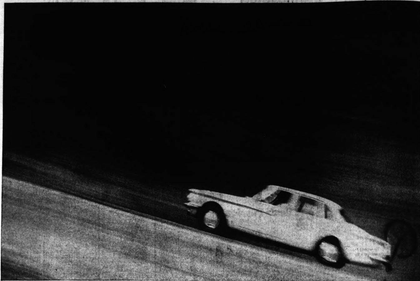
Shell experts test for knock by accelerating up steep grade. In another test, this "fifth wheel" in the back is lowered onto the road to measure mileage precisely.
