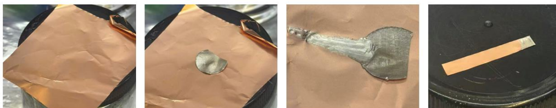
Figure 2.3 Preparation of the lithium counter electrode. (a) Preparation of the copper current collector. (b) Placement of a lithium foil on the copper current collector. (c) Lamination of the lithium foil onto the copper current collector to ensure good electrical contact. (d) Prepared lithium electrode after trimming to the desired dimensions. After both electrodes had been assembled, a glass coverslip was placed on top of the cell and bonded by heating the thermoplastic spacer to approximately 110 °C, forming a sealed optical chamber while leaving two openings for electrolyte injection. Approximately 40 \mu\text{L} of electrolyte was subsequently introduced through the openings, allowing the chamber to be filled by capillary action with minimal air entrapment. Finally, the injection ports were sealed using a two-part epoxy adhesive to prevent electrolyte leakage and solvent evaporation during electrochemical measurements. The completed optical electrochemical cell was then ready for in situ optical and electrochemical characterization.
