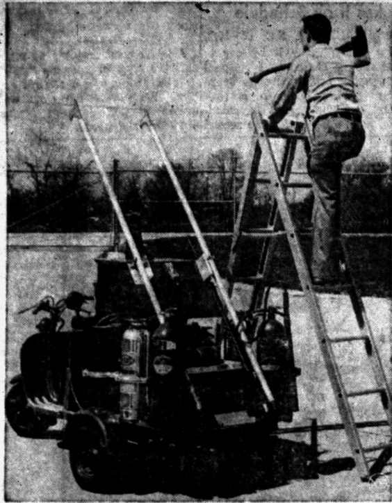
AT THE READY — A new method of providing instant protective measures in the case of fires or other emergencies is this vehicle announced by the Lofstrand Co. of Rockville, Md. Small and maneuverable, it can scoot through the aisle spaces of factories. Placed "at the ready" in strategic locations, it carries all necessary safety equipment, such as extension ladders, first-aid kits, resuscitator, gas mask, stretcher and fire extinguishers.
