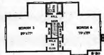
FLOOR PLANS: Center hall planning in both the front and rear is the key to excellent circulation in this house. Note also how the first floor sleeping area is set well apart from the entertaining area. Second floor can be finished a portion at a time as the extra space is needed.
