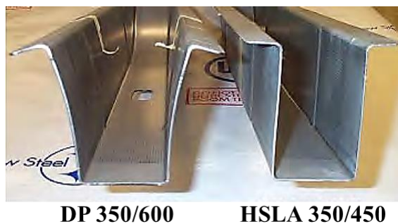
Figure 1.5. The springback difference between two channels made out of DP and HSLA steels [4].
