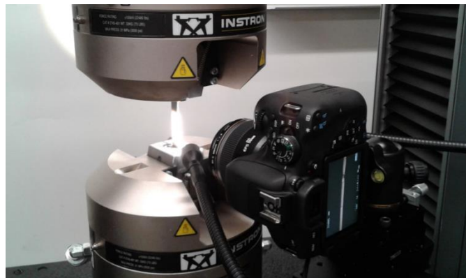
Figure 5.21. Tracking the fracture progression using a Canon T6i camera.
