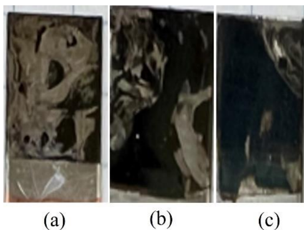
Figure 3.14: Sn-xSb sample prepared with solution 9 under different current densities: (a) 0.19 A/dm 2 , (b) 0.38 A/dm 2 , (c) 0.76A/dm 2
