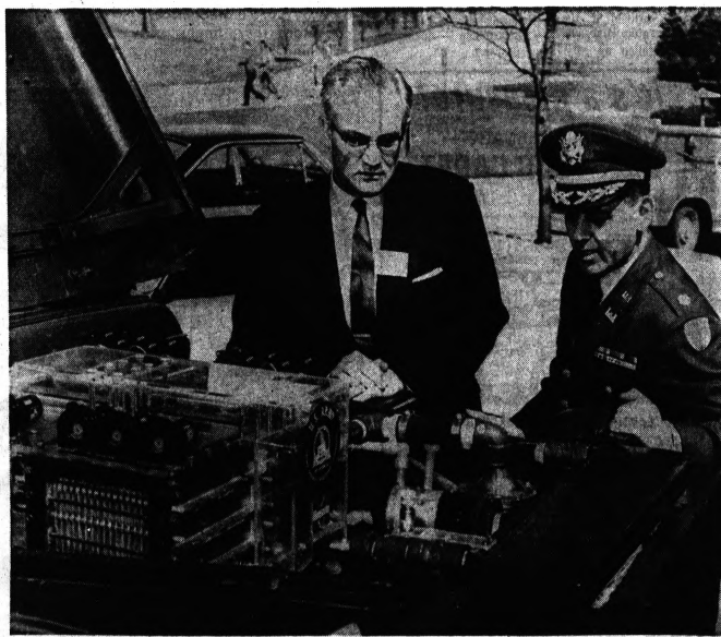
FUEL CELL TRUCK —Monsanto Research Corp. and the U.S. Army displayed in St. Louis, Mo., yesterday an electrically driven truck. The Army M37 truck has a gross weight of four tons and is powered by four fuel cells. In-
