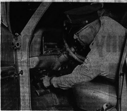
LIFESAVER —Oakland County Sheriff's Deputy Harold L. Hedges points to the energy-absorbing steering column he credits with saving his life in a recent collision. Hedges and Deputy Stephen M. Hubbell were on duty in a 1967 Pontiac in pursuit of a speeding car when the accident occurred. The column collapsed when Hedges was thrown against the steering wheel, thus absorbing much of the impact.
