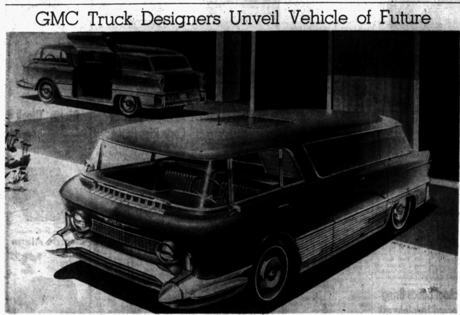
SLEEK AND USEFUL —GMC's all-purpose vehicle, L'Universelle, is this sleek panel delivery with front-wheel drive, V-8 180-horse-power engine, inverted hydraulic transmission, torsion bars, panoramic windshield and two-way radio-telephone. The grille for the air intake to the radiator is seen on the roof. Built by the GMC Truck & Coach Division, the GMC dream truck will be shown in GM Motoramas at New York, Miami, Los Angeles, San Francisco and Boston this year.
