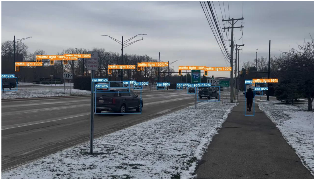
Figure 15. Representative object detection outputs from the cloud-based YOLOv8-small model using RSU camera footage during real-network trials. Vehicles, traffic lights, pedestrians, and other road users are detected with high confidence (typically greater than 95%). Bounding boxes remain stable and well-aligned, even during adaptive H.265 operation at reduced bitrate.
