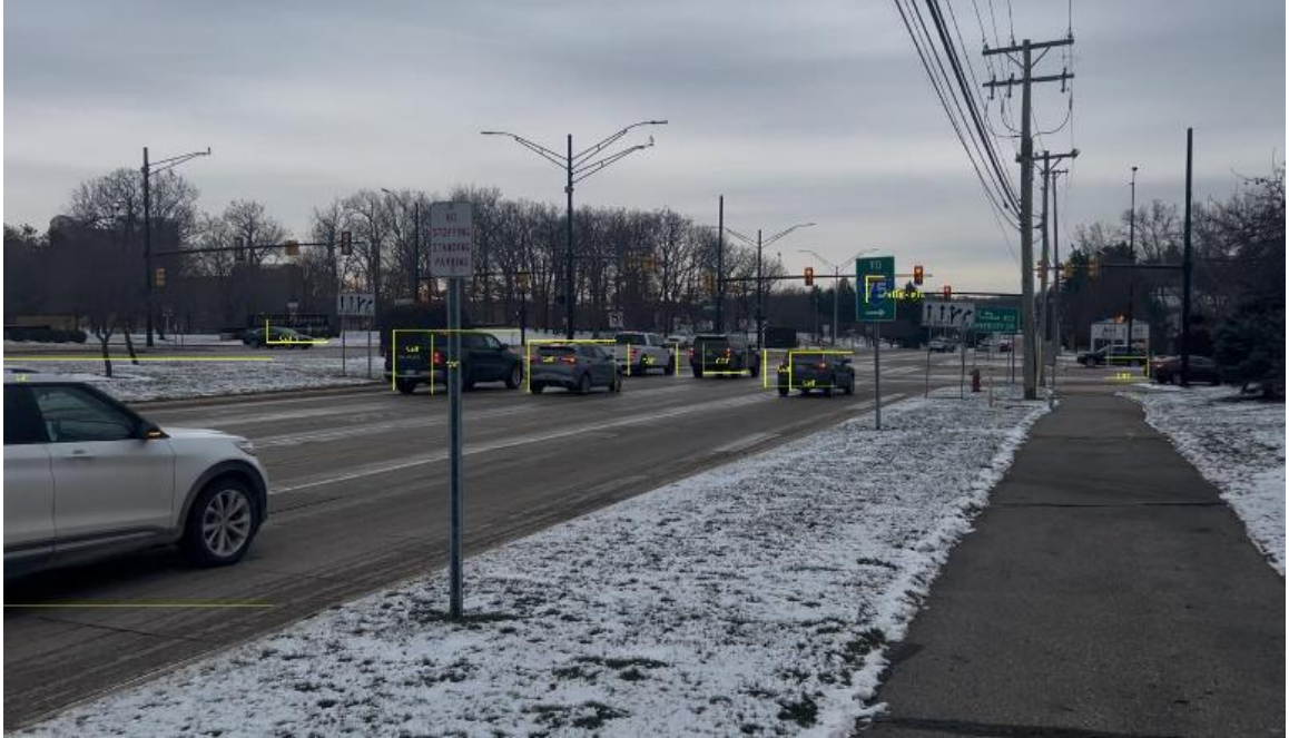
Figure 11: Example detection output from the YOLOv8-Small model using an RSU camera feed. Bounding boxes show detected vehicles under overcast conditions.
