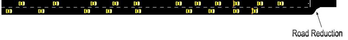
Figure 5.1: The AVs merging scenario in SUMO simulation environment, where each vehicle on the bottom lane is an RL agent. The goal is to learn an optimal merging strategy for each vehicle on the bottom lane so that the overall long term return is maximized. Note that the number of vehicles in the merging zone varies within a single episode, making the RL problem challenging as the number of agents is not fixed.
