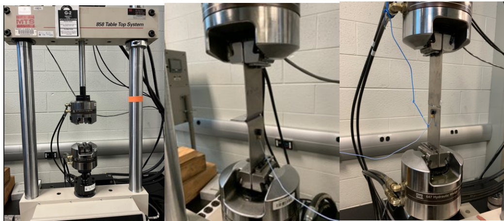
Figure 12. MTS 858 Tabletop System, Coach Peel and Lap Shear Samples Set Up
