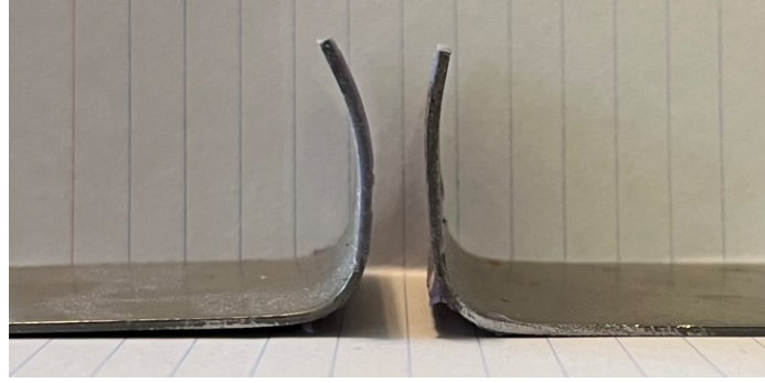
Figure 21. Bent Sheets for the Final Stage of Pull Test
