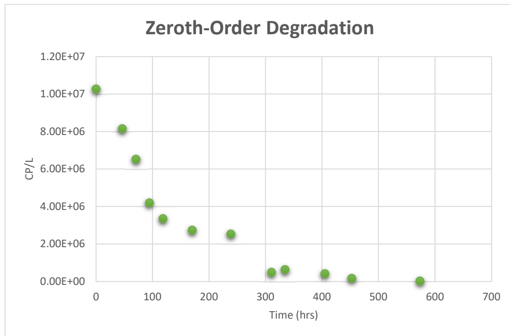
Figure 1.1: Reaction Order Example Based on One Sewage Sample
