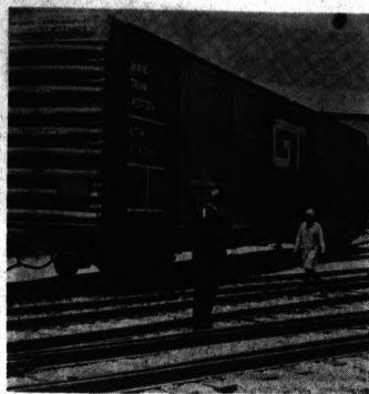
NEW EQUIPMENT —This is the first of 112 new 94-foot-long boxcars being made for Grand Trunk Western Railroad. With internal loading devices, they cost $38,000 each. They will be used by Chevrolet Division of General Motors.
