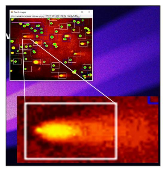
*Note*. The figure above describes the scanning step of the Comet Assay. White boxes are placed around comets that meet the programmed criteria for acceptance, while blue boxes are placed around potential comets that are not selected.
