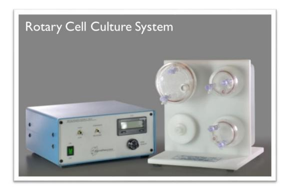
*Note*. The RCCS simulates microgravitational conditions.
