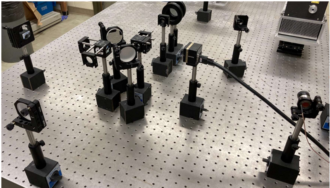
Figure. 6.6. The real setup of the dual sensitive shearography
