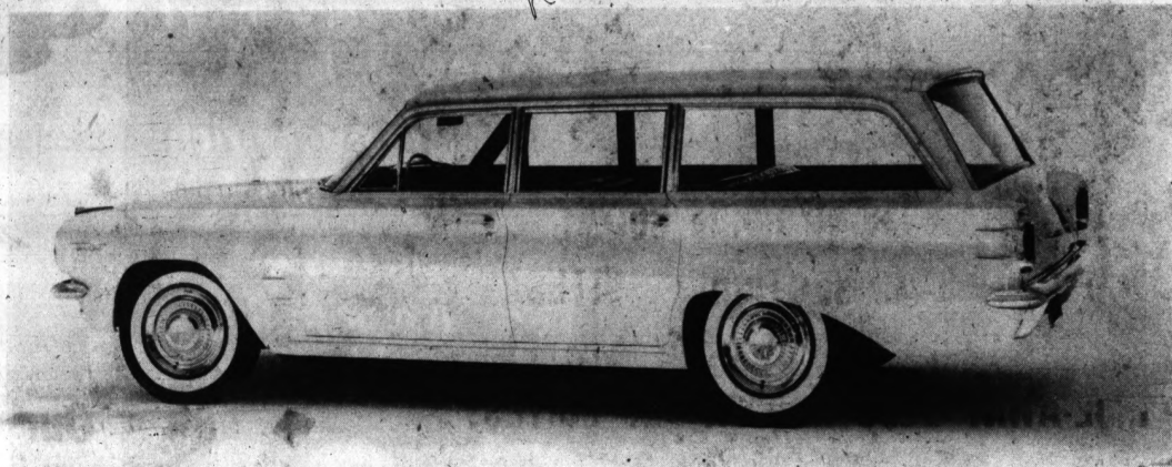
STATION WAGON FEATURES — Pontiac's Tempest station wagon is designed for comfort, economy and performance. Along with unit body construction and independent four-wheel suspension,
