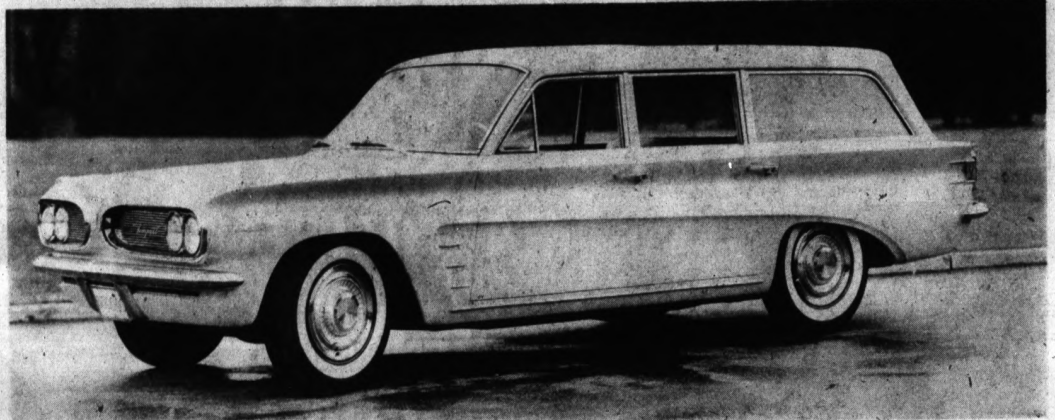
STATION WAGON FEATURES — Pontiac's Tempest station wagon is designed for comfort, economy and performance. Along with unit body construction and independent four-wheel suspension,
