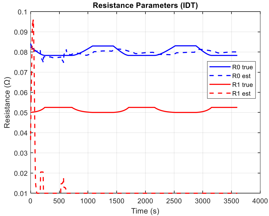
Figure 3.23. Time Evolution of Convergence of Estimated and True Resistances R_0 and R_1 (for IDT)
