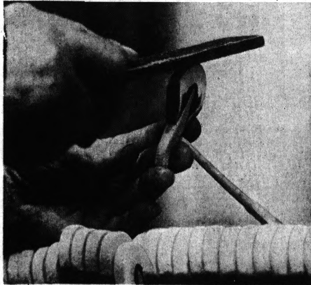
The hands of a master craftsman shape a hammer in an operation called "voicing," which creates a piano's tone. The stick is faced with sandpaper.
