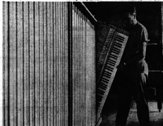
A workman inspects a set of 88 keys before inserting them in a piano. The "ivories" are no longer carved from ivory, but are manufactured from a more durable plastic.
