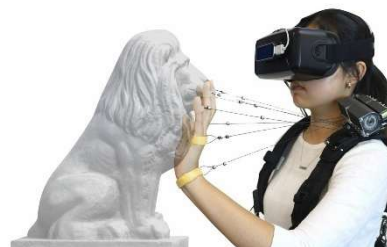
Figure 12- Wireality's Cable-based Brake Actuation
