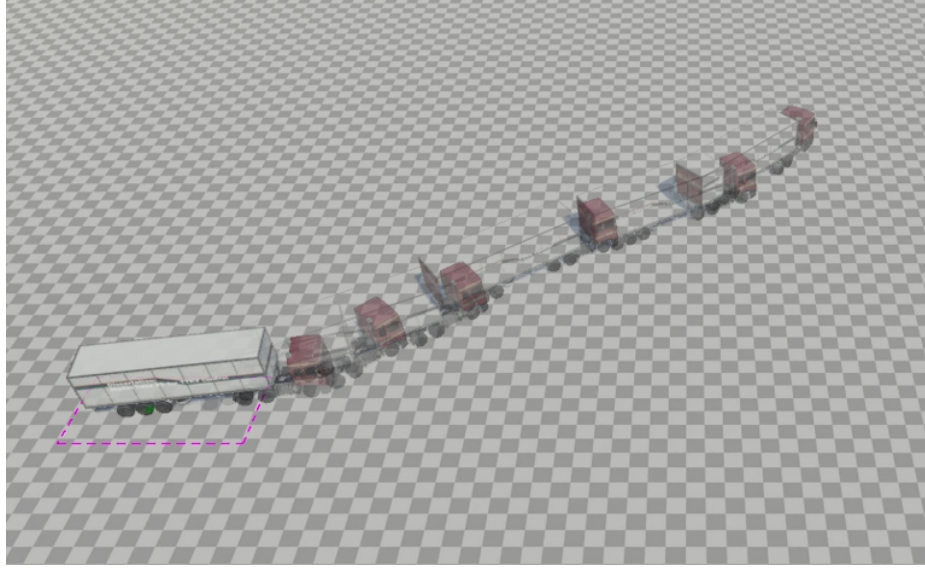
Figure 5.15: Unity visualization of trailer parking in obstacle-free environment using TD3WD.
