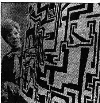
OP ART? — Not quite. It's a large-scale reproduction of the electronic circuit map printed on microminiature silicon chips produced by Westinghouse Electric Co. The final product, thousands of times smaller than this diagram, is an integrated circuit with thousands of uses in today's technology.
