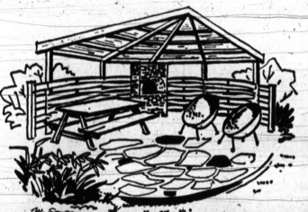
FOR ALL WEATHER —Barbecuing weather is all too short even in the most temperate parts of our country, but this cleverly designed, semi-enclosed roofed patio will add many weeks of outdoor living time each year. Light Douglas fir framing lumber and common boards form the roof with a simply woven half wall of one inch western red cedar boards.
