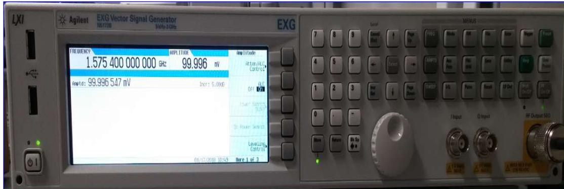
Figure 1.7: Photograph of generated RF sinusoidal wave at the RF output port of Agilent Technologies EXG Vector Function Generator 9 [kHz]-3 [GHz], signal center frequency =1.5754 [GHz], and signal amplitude= 100 [mV]
