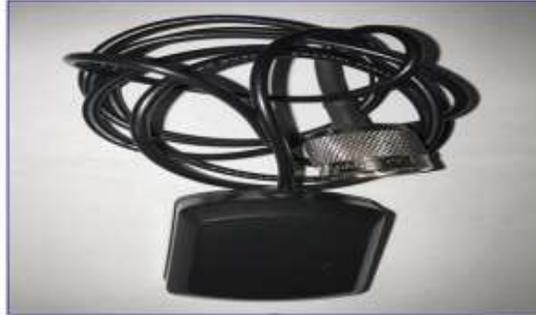
Figure 6. RF GPS Only Passive Patch Antenna
