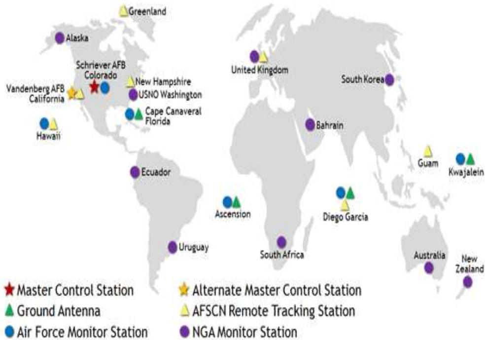
Figure 1.12: GPS control segment locations and facilities [56]
