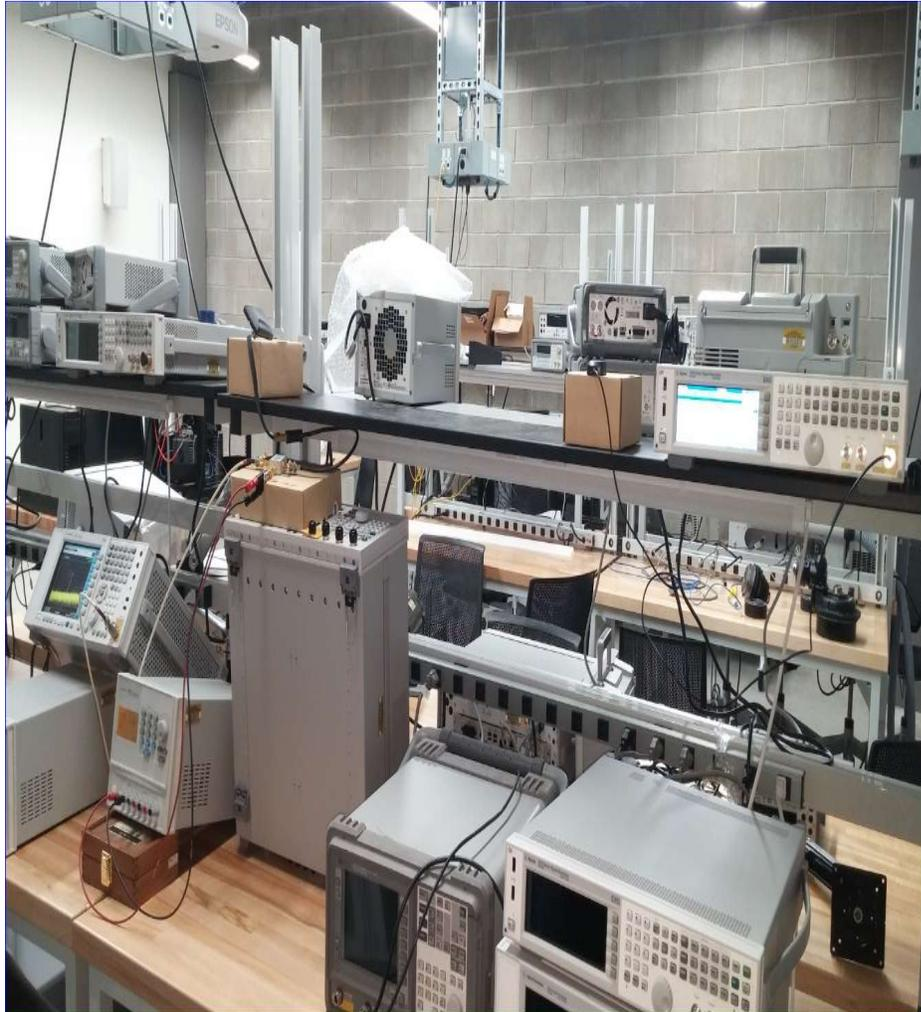
Figure 1.2: Photograph of transmit and receive mode instrumentation hardware antenna characteristic measurement setup
