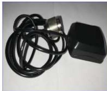
Figure 3. GPS Only Patch Antenna
