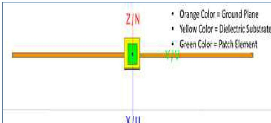
Figure 2.1: GNSS patch antenna operating at 1.555 [GHz] (Top View)
