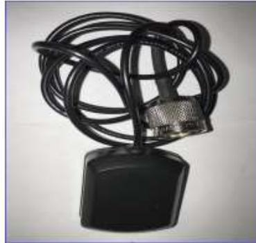
Figure 4. GPS Only Patch Antenna
