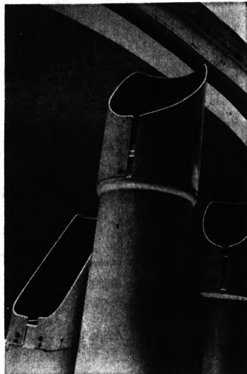
THREE EYES — That three barrels shoot better pictures than one appears to be indicated by the three-headed hydrogen patrol-flare telescope. Continually trained toward the sun, this telescope is standardized for international patrol of solar activity. Pictures of the solar disc are taken automatically at least every 30 seconds.
