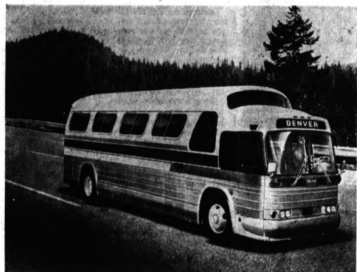
GMC BEAUTY — This new intercity bus, the "Luxury Liner," features high-level seating for maximum passenger visibility and greatly increased under-floor baggage space.
