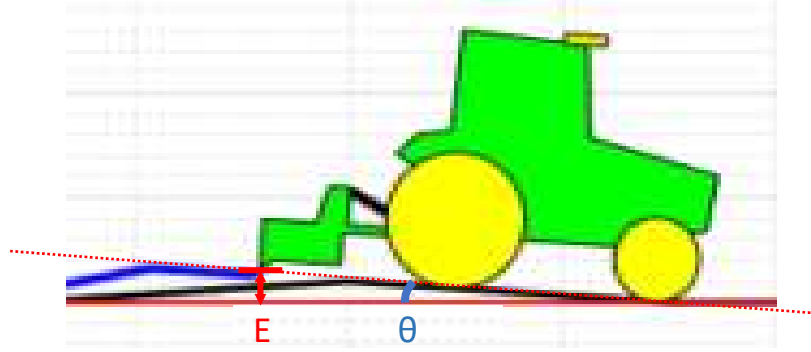
Figure 3.5: Tractor Ground Leveling Error
