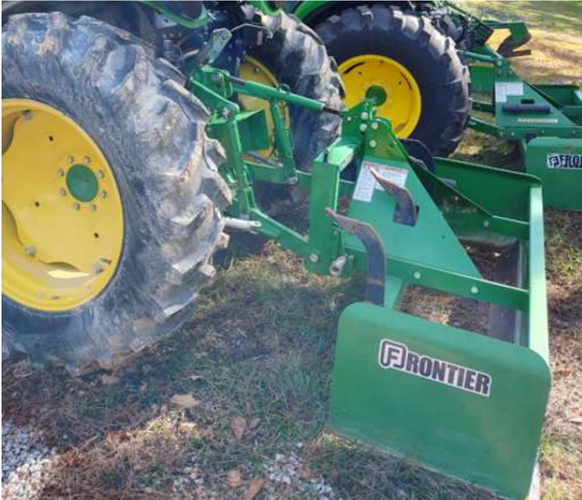
Figure 5.4: Tractor View After Rear Box Blade Attachment is Installed
