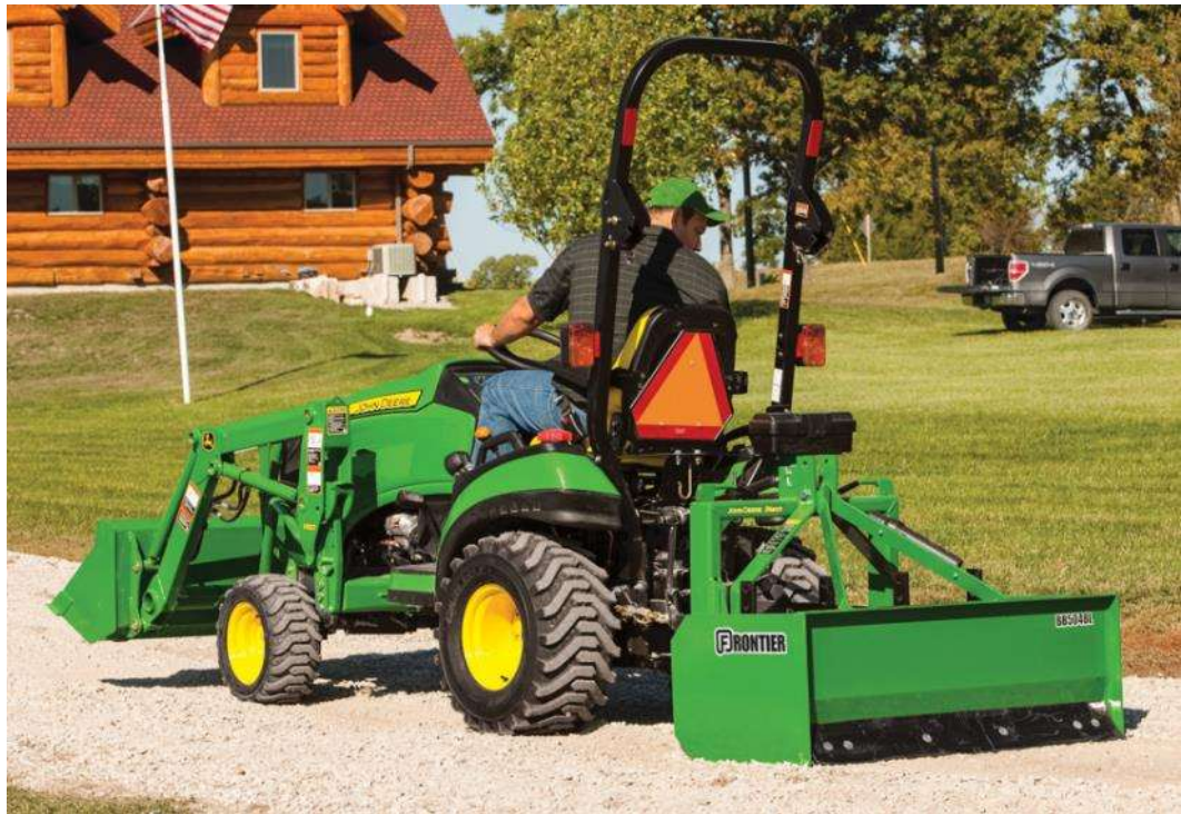
Figure 2.2: Tractor Ground Leveling Illustration [36]
