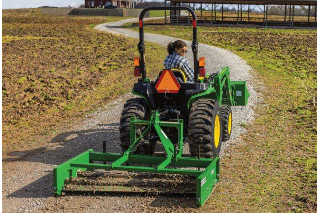
Figure 2.1: Tractor Ground Leveling Illustration [35]
